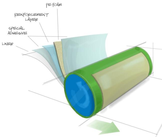
Special requirements are set to cross-linked, closed-cell polyethylene foams as carrier for cliché mounting tapes.
