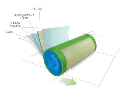
Special requirements are set to cross-linked, closed-cell polyethylene foams as carrier for cliché mounting tapes.
